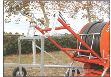
Automatic trolley hooking
