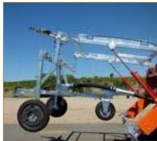
2000 series articulated trolley and hydraulic lifting frame
