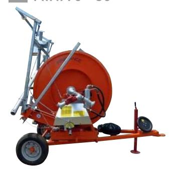
Featuring a low-speed turbine flanged on gear box, this machine operates from 4 m3/h with a low pressure drop it offers optimized performance.
